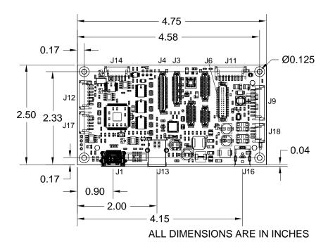
Notes: Tallest component top side is 0.45". Printed circuit board thickness 0.062"  $\pm 10$ %. Tallest component bottom side is 0.075".
